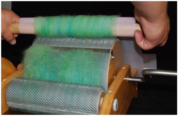
Roll the Batt Lifter away from you while keeping the Batt Lifter in contact with the teeth of the large drum. The large drum of the carder will roll towards you as you roll. Staying in contact with the teeth will ensure that you remove as much of the fiber as possible.
