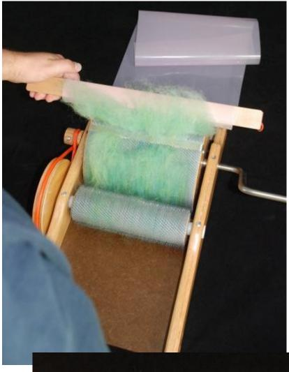
Unroll the Batt Lifter and slip the bands off the ends. You will have two pieces of wood: One with the antistatic sheet and one without. While standing in front of the carder- with the tray closest to you and the drums away from you place the anti-static sheet on the far side of the large drum with the flat half of the wood facing you. With the other piece of wood, sandwich the tips of the fiber on the ends of the batt farthest away from you, between the two wooden pieces.
