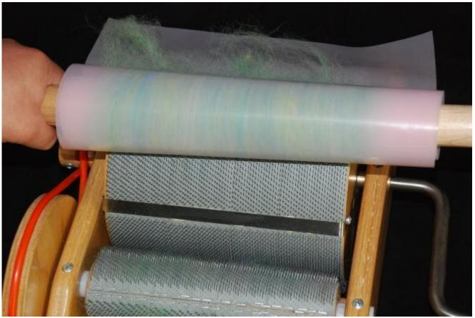
When you have rolled the entire batt off of the large drum continue to roll until the anti-static sheet is wrapped completely around the batt. At this point you can either unroll the batt for more carding or blending or you can store your batt for later use. To store it, slip the entire package (Batt Lifter with the anti-static sheet and fiber enclosed) inside the clear tube.
