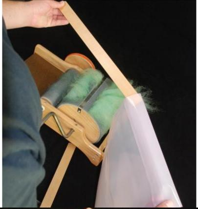
Slip one of the pieces of wood into the pocket of another anti-static sheet and you are ready to lift another batt.
