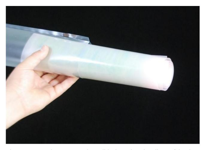
When you are ready to use your batt, slide the anti-static roll out of the clear plastic tube and unroll it.
